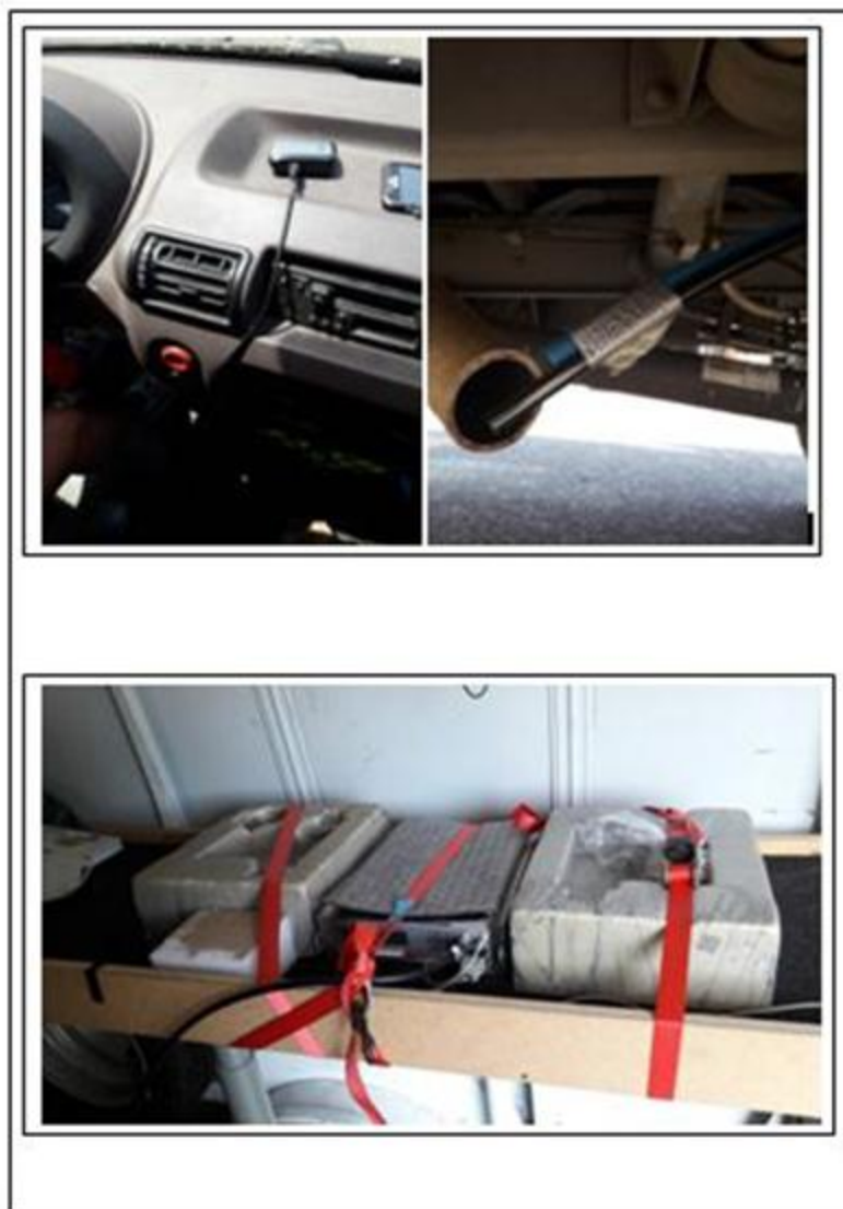
Figure 3. 2: Field study set-up (Exhaust emissions)
